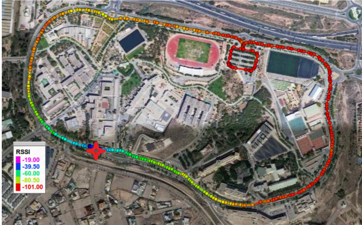
Figure 5: Heat map representing the level of RSSI received by the moving vehicle in the V2V scenario within the university campus. The red star represents the stopped vehicle.
