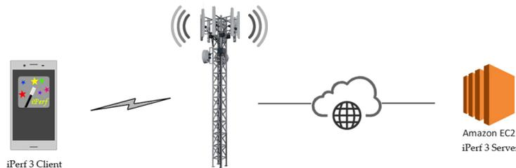
Figure 7: iPerf 3 measurements testbed
