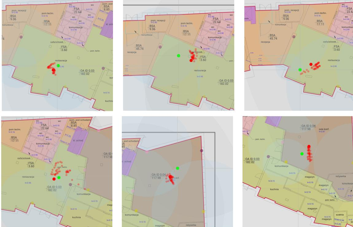
Figure 9: Measurements for 6 sample locations with filtering, smoothing and centroid calculations (large red dots, green dots represent real positions).
