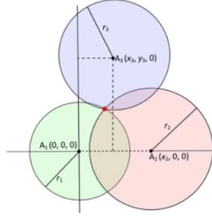
Figure 3: Local coordinate system for a sample trilateration problem [27].
