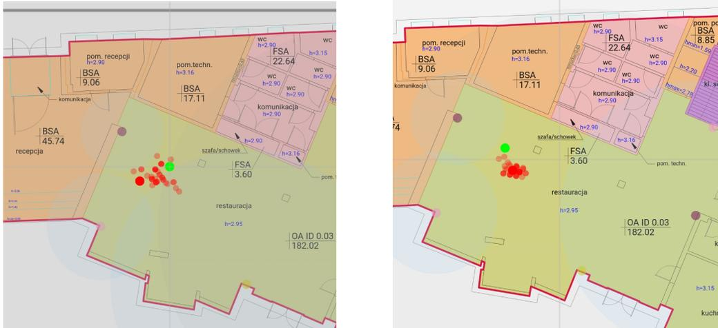
Figure 8: Computed positions (red dots, green dots represent the real positions) before and after signal smoothing.
