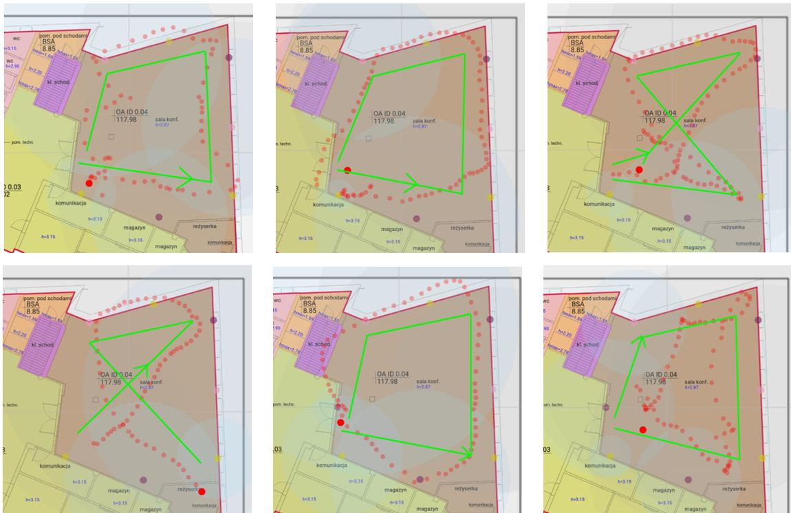
Figure 11: Computed positions of a moving object (red dots) vs. real movement trajectories (green polylines) with increased number of beacons.
