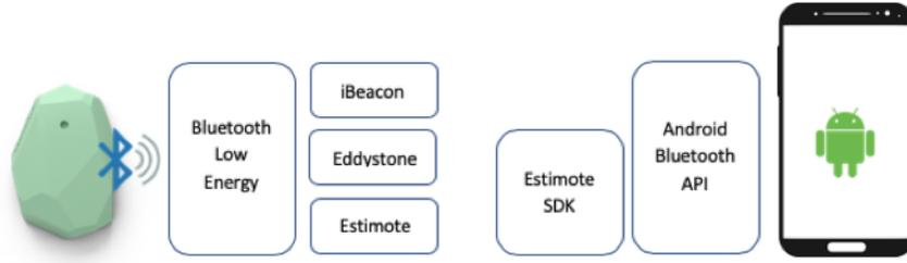
Figure 2: Estimote beacon communication schema.
