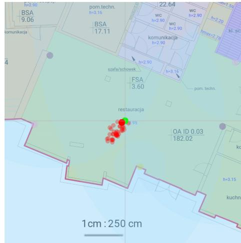
Figure 5: Floorplan with the real position marked green and 40 taken measurements marked red.
