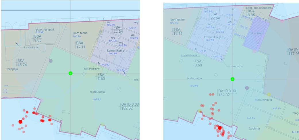
Figure 6: Negative effect on the measurements resulting from including weak signals from beacons located in other rooms.
