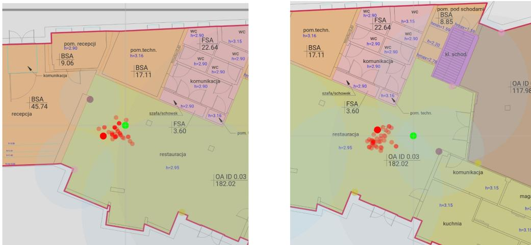
Figure 7: Computed positions (red dots, green dots represent the real positions) after filtering out weak beacon signals.
