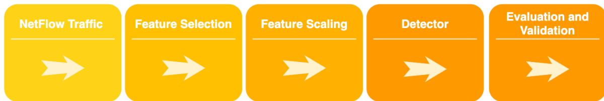
Figure 4: The flow-based real-time machine learning network intrusion detection data processing pipeline
