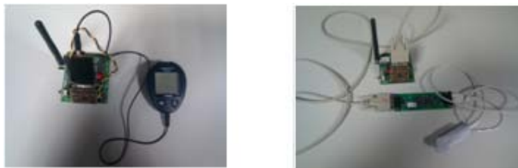
Figure 3: Mobile sensors connected trough 6LoWPAN
