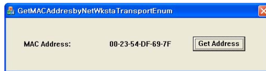
Figure 7: Result of the implementation using NetWkstaTransportEnum
