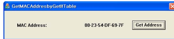
Figure 11: Result of the implementation using GetIfTable function
