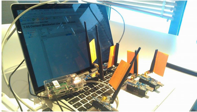
Figure 15: RPi running 6LBR, connected over USB to the slip radio and via Ethernet to a development PC and the various sensors running CoAP servers
