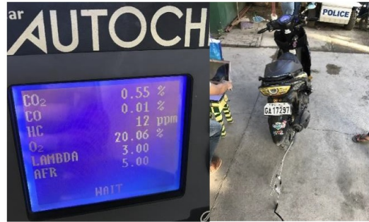
Figure 11: PETC's measurement using Authocheck TM Exhaust Gas Analyzer
