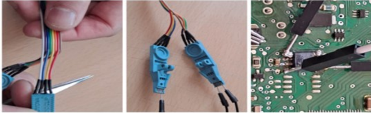
Figure 6: Manufacturing process of a serial communication cable and connecting it to the EEPROM
